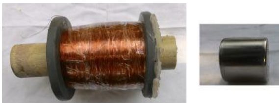
Figure 4. Linear generator system with Neodymium Magnets
