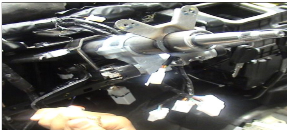
Figure 9. Steering lever opened for product left side bolt (Open condition)
