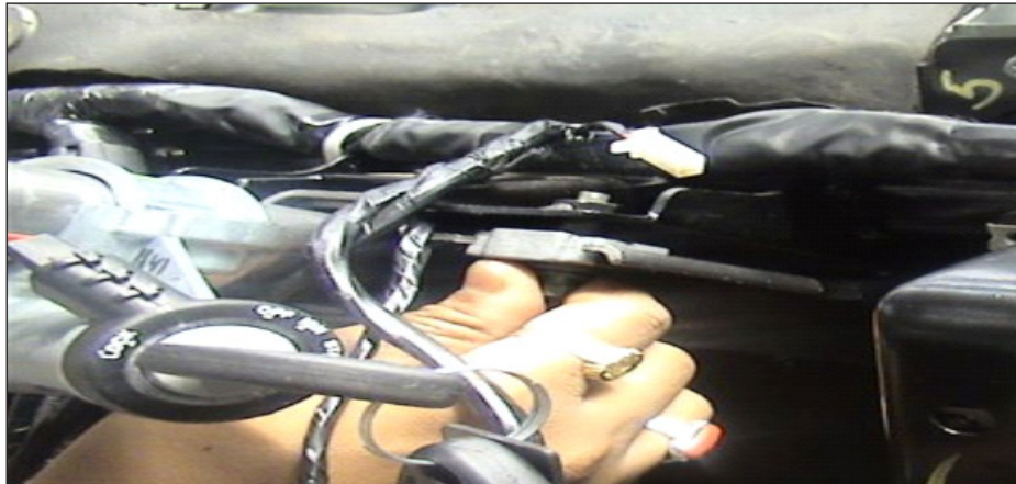
Figure 8. After placing Steering column on dash panel right side bolt of CCB is pre
