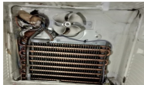
Figure 2.Evaporator chamber of refrigerator
