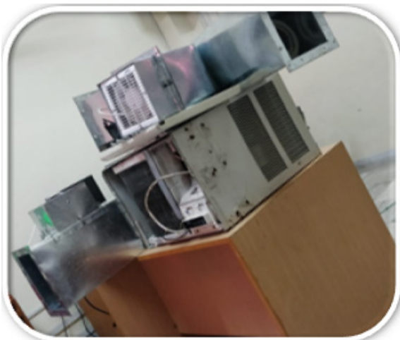
Figure 3. Duct assembly for window ac
