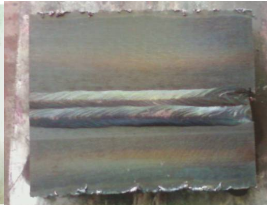
Figure 3. Weld bead after removing excess penetrant
