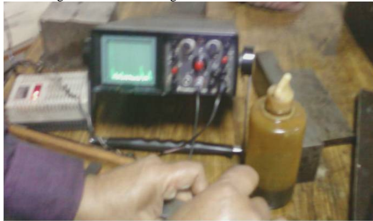
Figure 7. Ultrasonic test is being conducted on weldment
