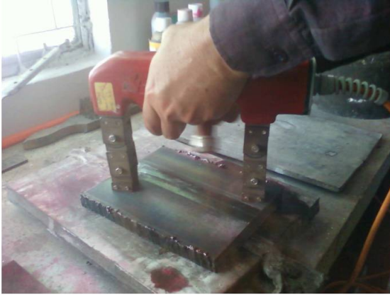
Figure 5. Material magnetized by applying yoke
