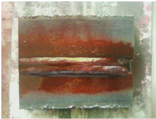
Figure 2. Penetrant applied on weld bead
