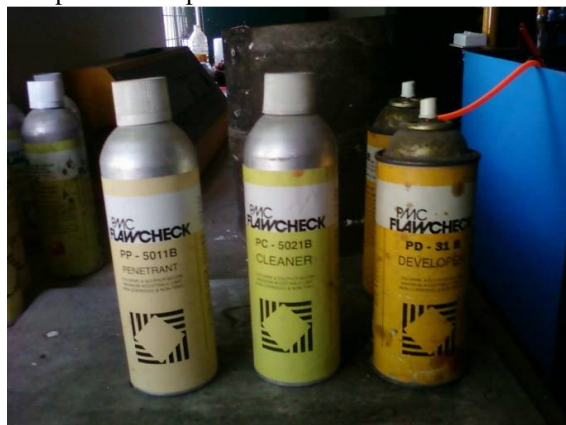
Figure 1. Ingredients of Dye penetrant test
