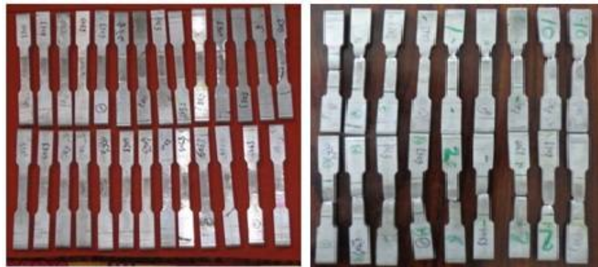
Figure 1. Tensile test specimens before and after test
