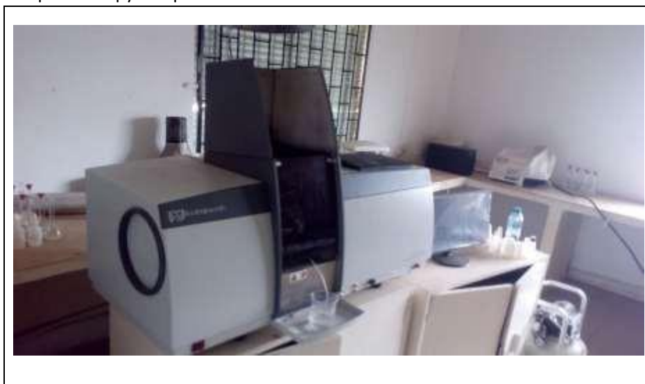
Figure 6: Atomic absorption spectroscopy (AAS) setup
