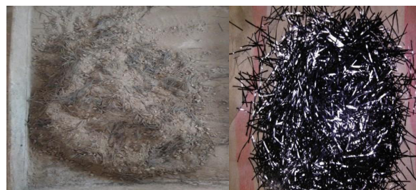
Figure 4. Randomly Distributed Carbon Fibres Three-point flexural test
