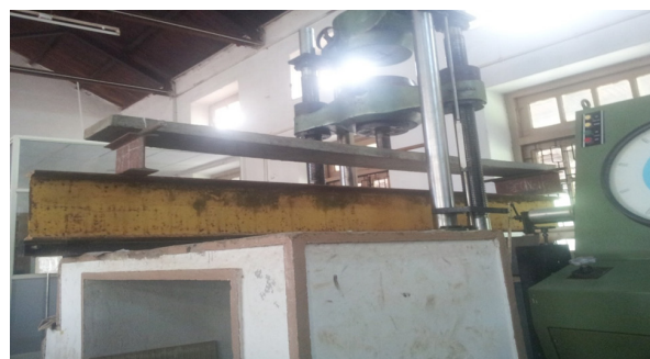
Figure 5. Load setup for single point loading Result and Discussion
