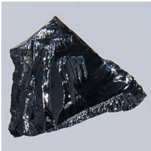
Figure 2. Silicon crystals are the most common semi-conducting materials used in microelectronics and photovoltaics
