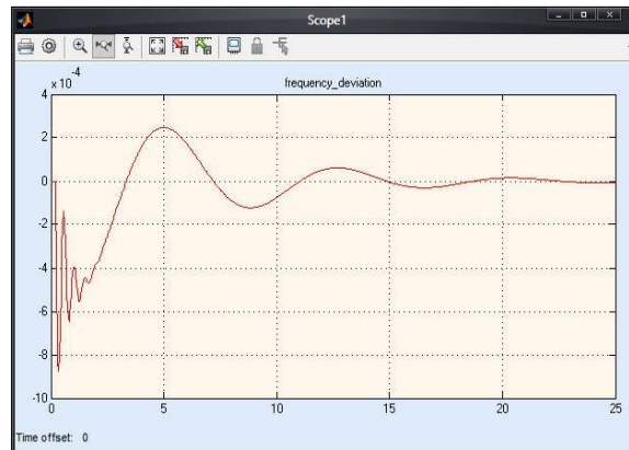
Figure 16 (d).Zoom View of Step Response of Generator-load Frequency Deviation with TLBO based PID Secondary Control Loop
